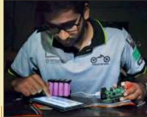
➤ Raspberry Pi being used as the dashboard for display of RPM & Battery Management System Data
