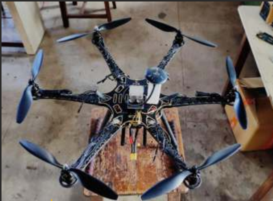
Drone Cleo assembled with all the electronics and components installed to test the Algorithms developed by the AI Team
