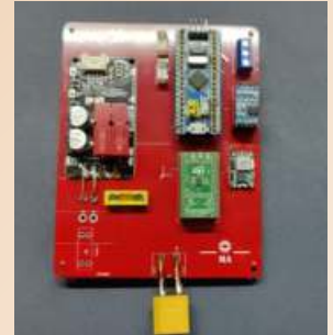
➤ STM&IMU integrated PCB for robotic manipulator
