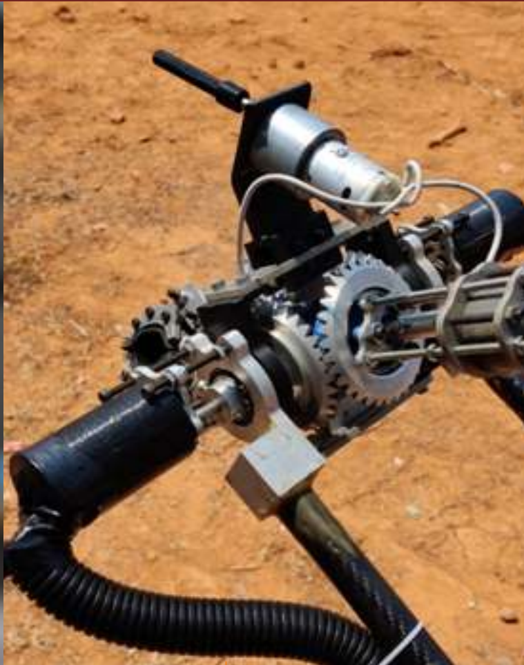
➞ A bevel differential powered End Effector
