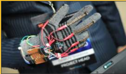
Talking Glove: With the heart of gold and the arm of code, the Talking Glove lends a helping hand towards the deaf. It works on a fundamental idea- to convert gestures and signs into a speech output.
