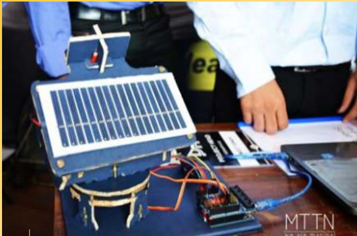
Dual Axis Solar Tracking: The Dual Axis Solar Tracking Panel automatically configures itself in response to lighting and weather conditions to receive an optimal amount of solar energy to be generated into electricity.
